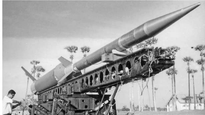
A Nike-Apache two-stage rocket on its launcher at Thumba, Kerala. THE HINDU ARCHIVES
